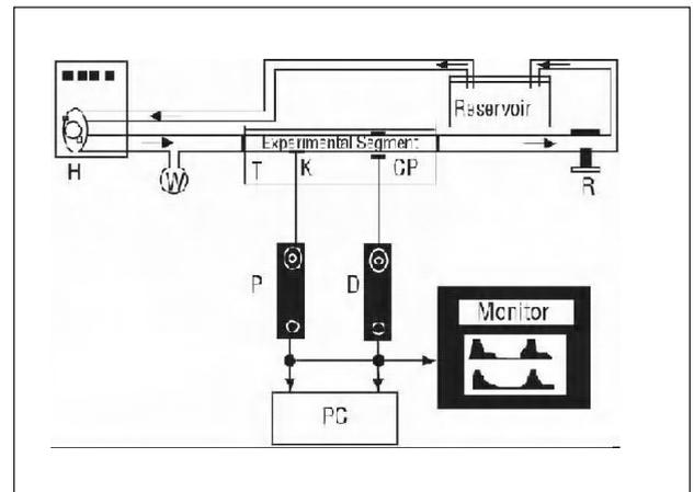
**Figure 2.** In vitro system. H indicates pneumatic pump and artificial heart; K, pressure sensor (Konigsberg); GP, diameter sensor (ceramic piezoelectric); P, pressure signal; D, diameter signal, and PC, computer. Arrows indicate the direction of flow. T, container filled with Tyrode's solution. Reservoir contains Tyrode's solution. W indicates a distensible chamber. R indicates a flow resistor.
