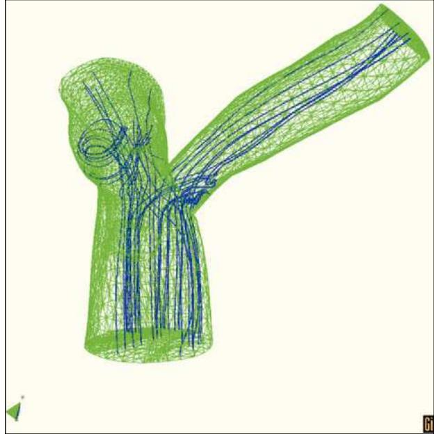
Figure 6. Three-dimensional T model with the predicted the trajectory of the particles.
