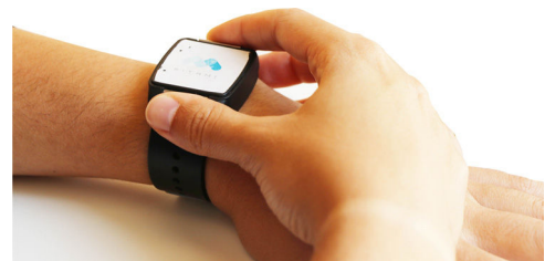
Figure 1. Position of heart rhythm monitor and placement of thumb and index finger to record the electrocardiogram.
